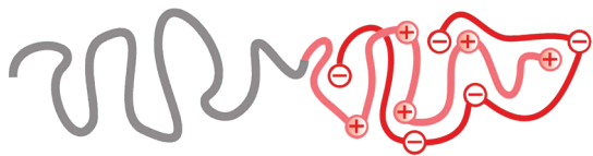
Figure 1. Sketch of diblock copolymer comprising nonionic and ionic blocks. Oppositely charged linear chain forms complex with the ionic block.
